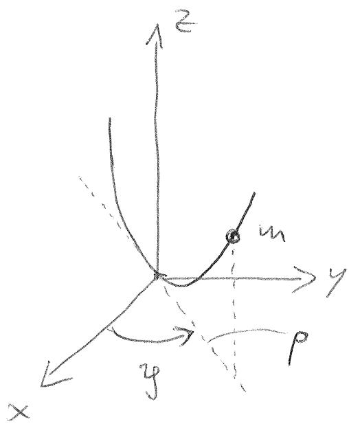
$$\begin{aligned} \text{zB } y - \omega t &= 0 \\ z - \alpha p^2 &= 0 \end{aligned}$$
