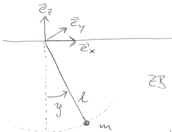
$$\begin{aligned}\text{ZB: } & x^2 + z^2 = l^2 \\ & y = 0\end{aligned}$$
