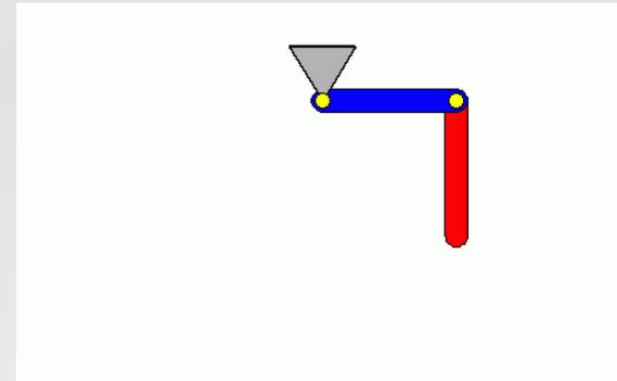
$$(m_1 + m_2) l_1 \ddot{\varphi}_1 + m_2 l_2 \ddot{\varphi}_2 \cos(\varphi_1 - \varphi_2) + m_2 l_2 \dot{\varphi}_2^2 \sin(\varphi_1 - \varphi_2) + g(m_1 + m_2) \sin \varphi_1 = 0$$
