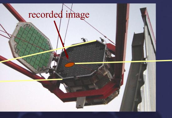
**Fig. 1b:** Each H.E.S.S. camera consists of 980 photomultiplier tubes and a fast read-out electronic.
