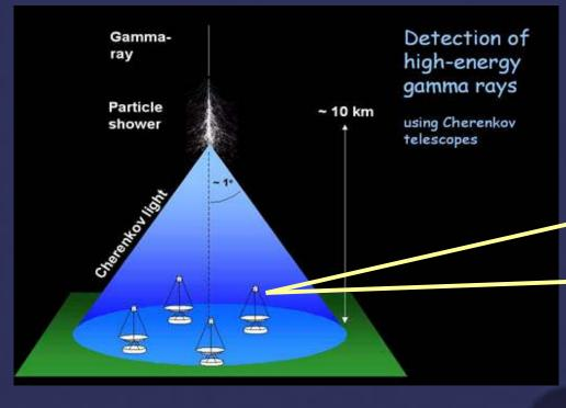
**Fig. 1a:** The Cherenkov light of an extended air shower is recorded by the H.E.S.S. telescope cameras.
