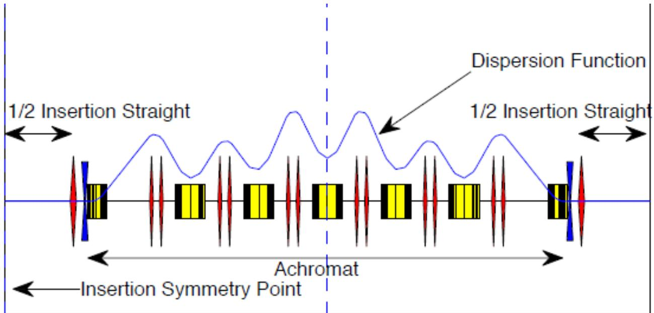
In order to save space, the unit cells have defocusing bending dipoles!
