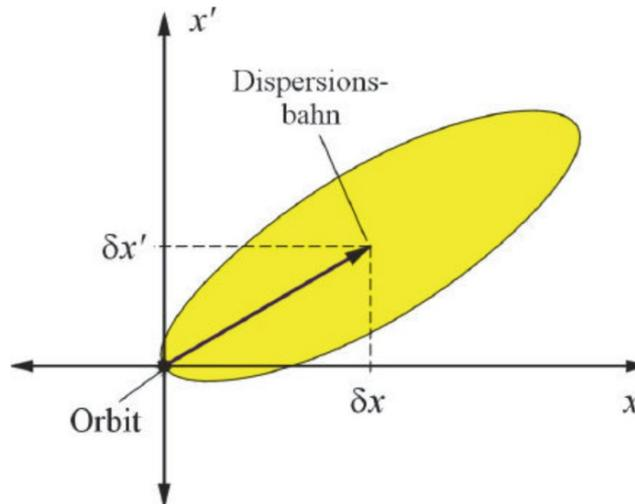
The excitation results from the increase of the horizontal oscillation amplitude
