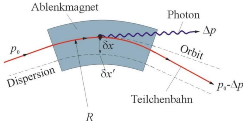
As a result of the variation of the particle's energy the betatron amplitude increases. The easiest way for its determination is the determination for one particle circling before the emission with design momentum on the design orbit. After the emission it is resided on a dispersion orbit with
