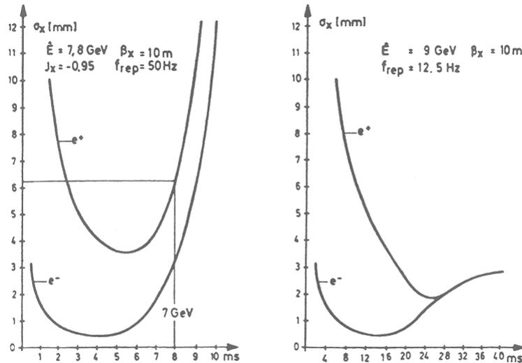
Variation of horizontal beam size with time during the acceleration cycle in the DESY I (left) and DESY II (right) synchrotrons [24]
