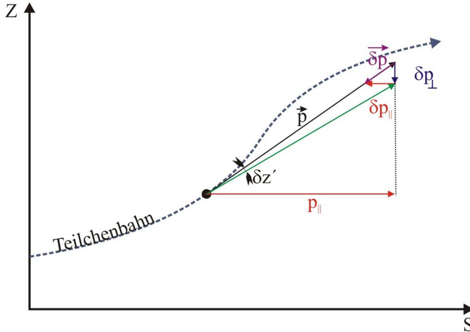
So, the small angle  $z'$  of the particle's momentum is decreased with respect to the  $s$  axis for the absolute value
