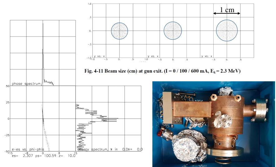
Fig. 4-10 Energy (KeV) and phase (deg.) (=length) distribution at the gun exit. (I = 600 mA,  $E_k$  = 2.3 MeV)
