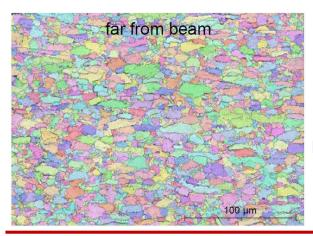
main grain area [ $\mu$ m<sup>2</sup>]: 19  $\mu$ m<sup>2</sup> (far beam area) 50  $\mu$ m<sup>2</sup> (far beam area)
