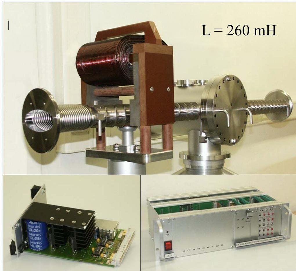
Beam pipe optimized for eddy current suppression
