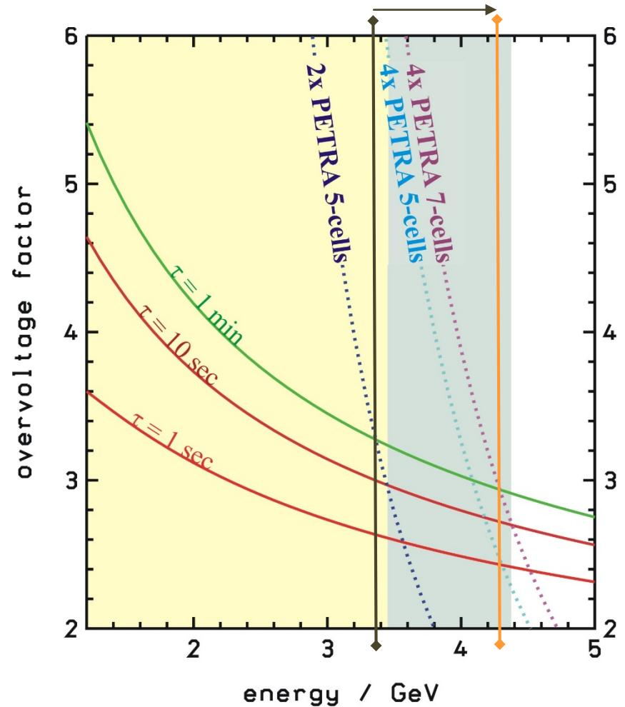
with four 7-cell resonators  $E \leq 4.3 \text{ GeV}$  @  $\tau = 1 \text{ min}$
