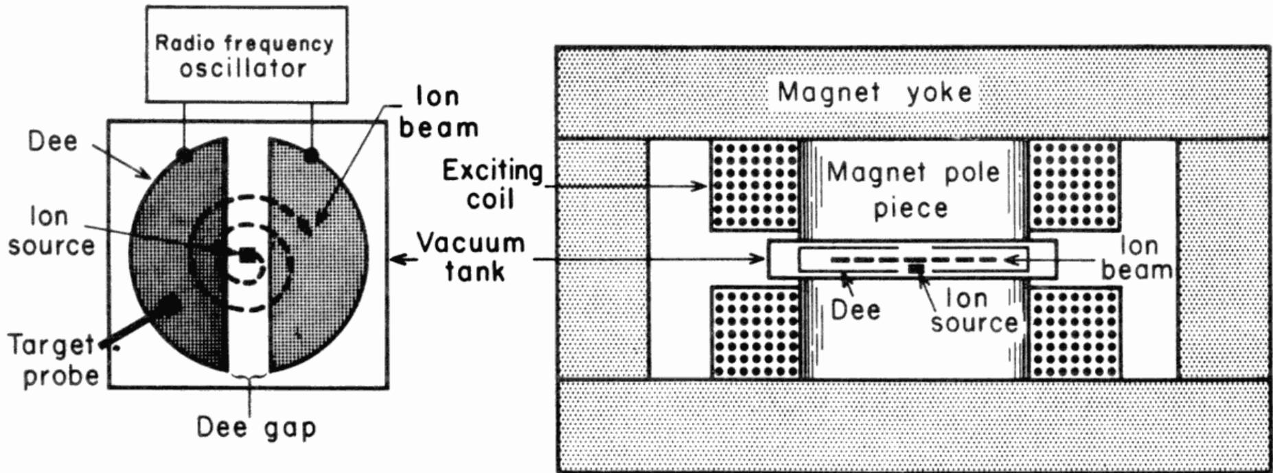
We employ an “isochronous cyclotron” design where the magnetic field changes with radius. This can accelerate many bunches at once.
