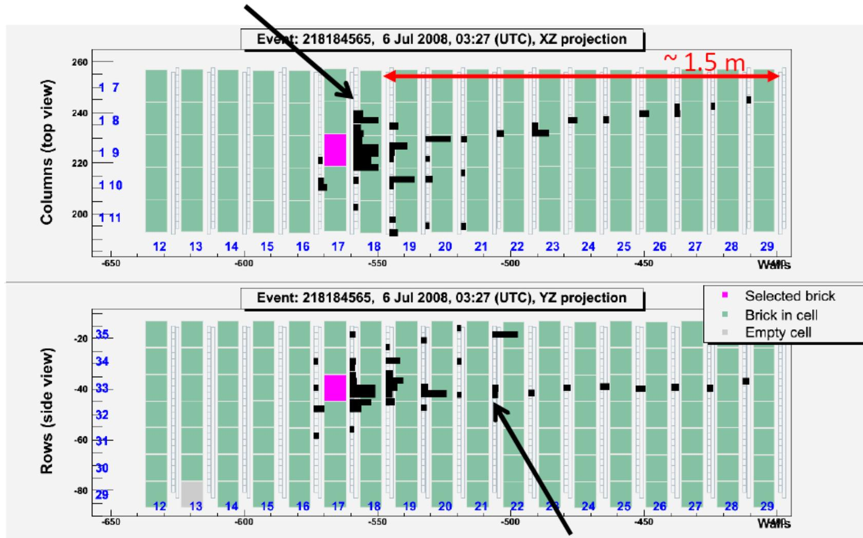
Track identified as a muon ( $P=3.394 \text{ GeV}/c$ )
