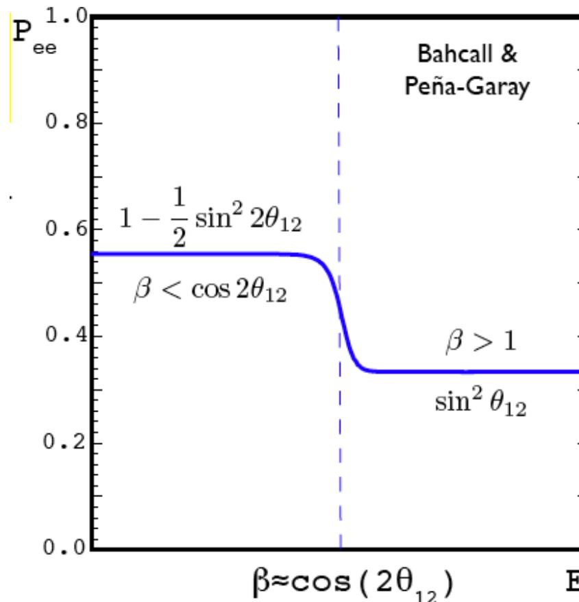
$$\beta = \frac{2^{3/2} G_F N_e E}{\Delta m^2} = 0.22 \left[ \frac{E}{1 \text{ MeV}} \right] \left[ \frac{\rho \cdot Z/A}{100 \text{ g cm}^{-3}} \right] \left[ \frac{7 \times 10^{-5} \text{ eV}^2}{\Delta m^2} \right]$$
