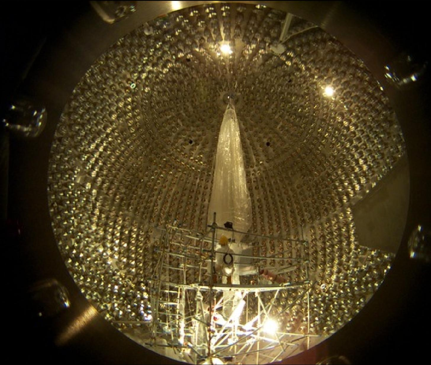
Installation of the 2 inner nylon spheres
