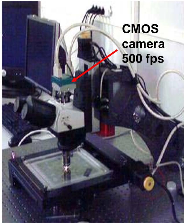
Final version of the european system ready and working at 20 cm<sup>2</sup>/hour (15 stations under installation)
