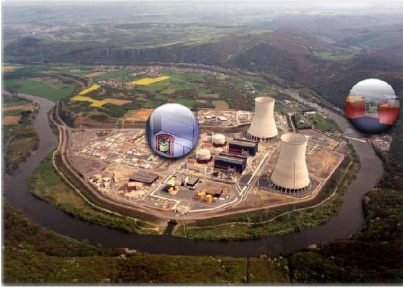
Figure 3.1: The Chooz reactor plant with positions of DoubleChooz near and far detectors.
