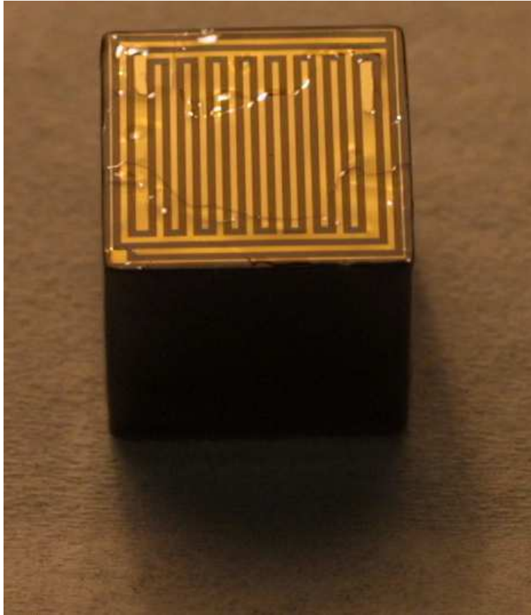
Figure 3.2: Picture of the coplanar grid design of a colorless passivated 1 \text{ cm}^3 CdZnTe detector [COB].
