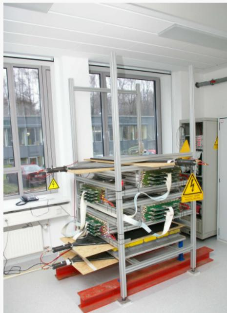
Each module consists of 48 aluminum drift-tubes.
