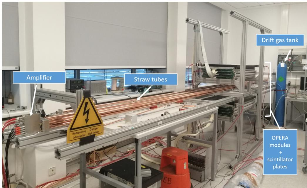
Figure 5.1: The test station including straw tubes, OPERA modules, drift gas tank and amplifier. The readout electronics are located on the left. The straws have a length of 5 m.
