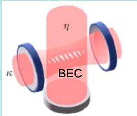
$$H = -\Delta_C a^\dagger a + \int_0^L \Psi^\dagger(x) \left[ -\frac{\hbar}{2m} \frac{d^2}{dx^2} + U_0 a^\dagger a \cos^2(kx) + i\eta_t \cos kx (a^\dagger - a) \right] \Psi(x) dx,$$
