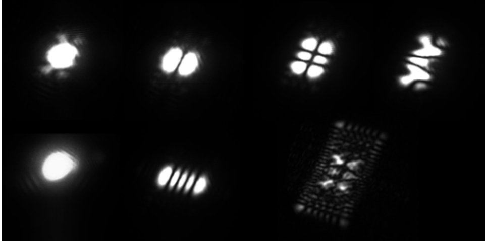
Figure 5.7 – On the left the TEM_{00} mode is shown in the unlocked (top) and locked (bottom) case, the contribution from higher order modes are clearly visible in the upper picture. Beside the shown higher order modes ( TEM_{10} , TEM_{12} and TEM_{40} ) many strange transversal modes were lockable where two examples are shown on the right.
