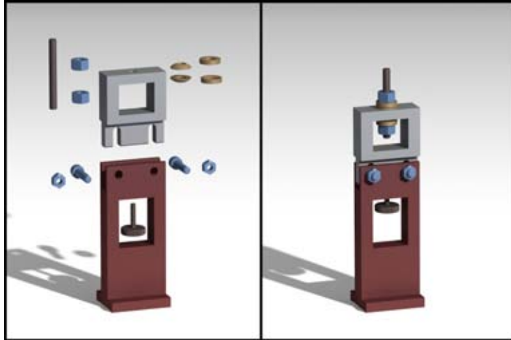
Figure 3.10 – These mountings were developed to ensure a stable chamber mounting and the possibility to assemble the magnetic coils after the bake-out. First the threading stick will be placed in special bores in the bottom of the main chamber. Then the upper part of the mount will be mounted and finally the chamber can be fixed on the optical table with the lower part of the mounts where the upper part is tightly clamped by the two vertical screws.
