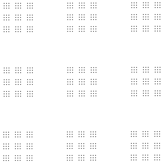
Fig. 11.15: Concatenated quantum coding in an optical lattice. At each coding level, two-dimensional lattice displacements with an increasing periodicity are applied. The nested character of Fig. 11.14 is here reflected by a self-similar filling pattern of the lattice.
