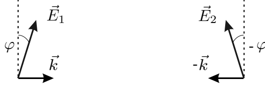
Fig. 12.3: Laser configuration for a state selective optical potential. Two standing circular polarized standing waves are produced out of two counterpropagating running waves with an angle 2\varphi between their polarization axes.
