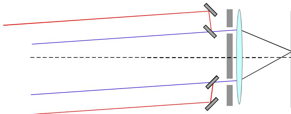
Michelson stellar interferometer: adjustable slits, extension of slit separation by mirrors
