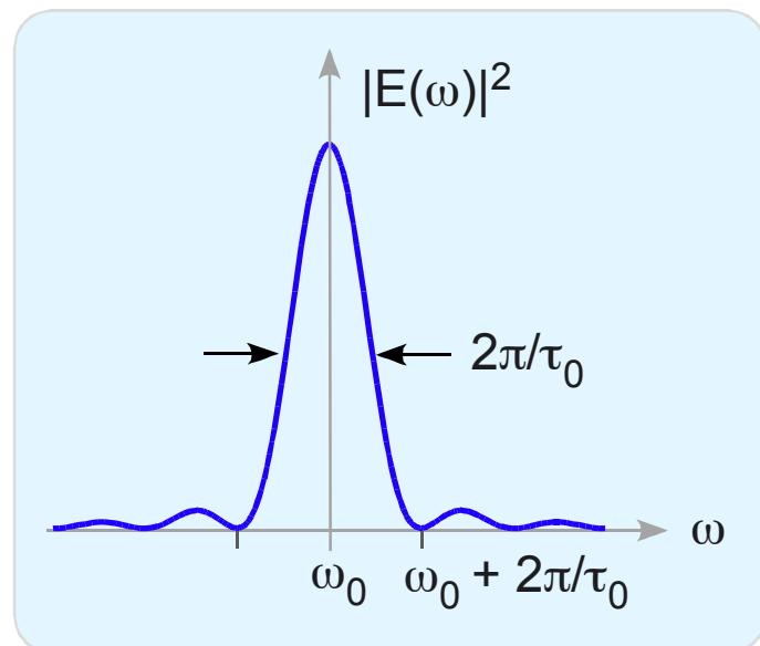
$$E(\omega) = \sum_{n=1}^N \sqrt{\frac{2}{\pi}} \frac{\sin[(\omega - \omega_0)\tau_n/2]}{(\omega - \omega_0)} \exp(i(\omega - \omega_0)t_n - i\phi_n)$$
