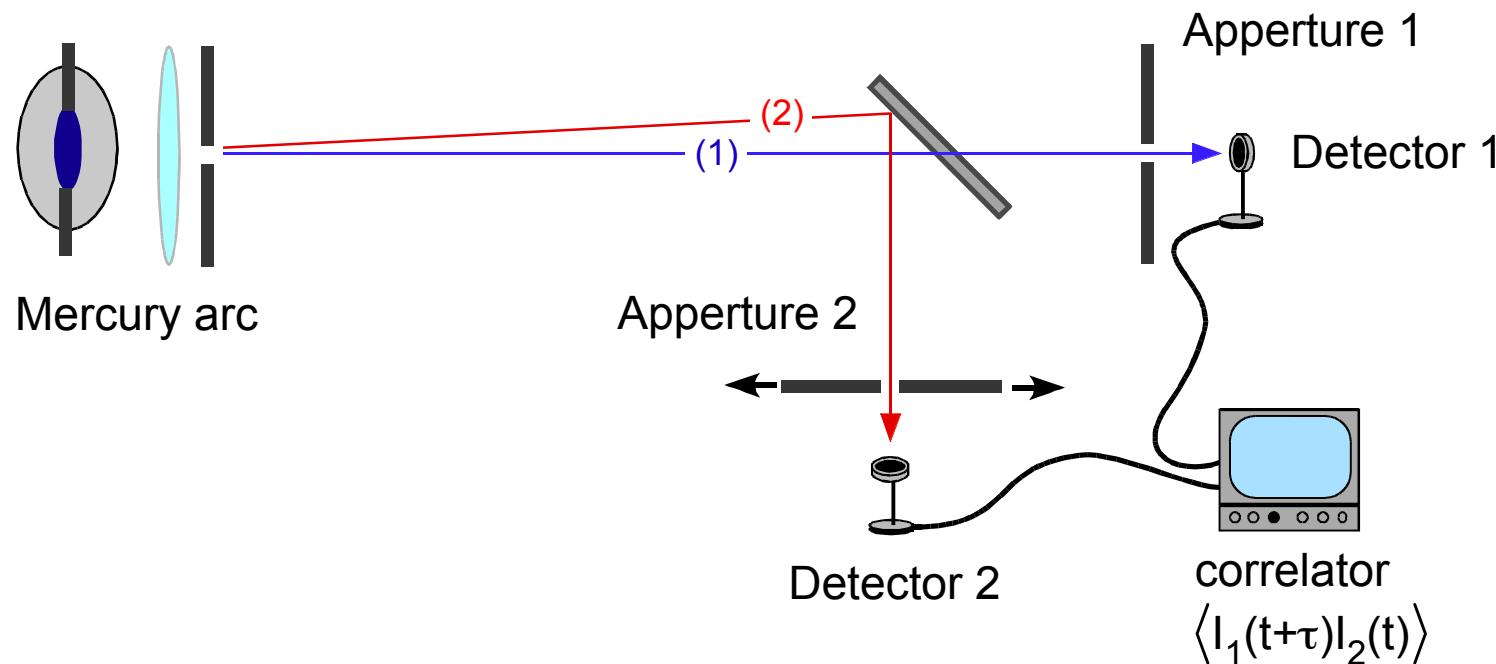
Variation of aperture 2 permits measurement of transverse coherence length
