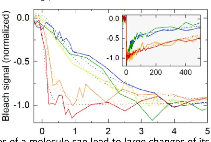
collodial HgTe QDs studied by femtosecond infrared pumpprobe spectroscopy.
