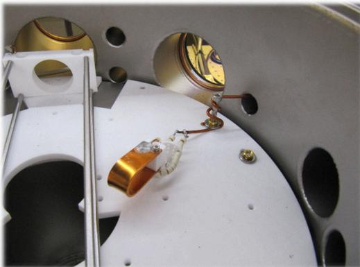
(c) Microwave antenna as inspired by [142]. A Kapton isolated coaxial line is soldered to an OFHC loop located in the vicinity of the experiment position.
