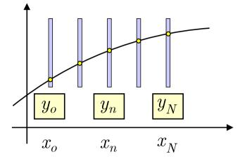
The detectors are placed at positions  $x_0, ..., x_n, ..., x_N$ A track crossing the detectors
