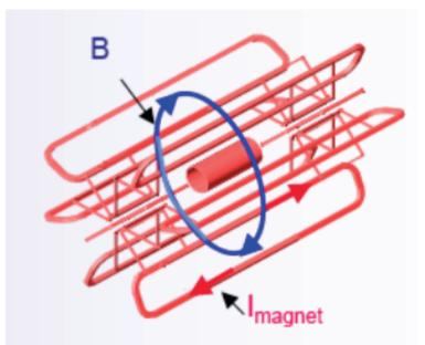
Example: •ATLAS: Barrel air toroid, SC, ~1 T, 9.4 m, L 24.3 m
