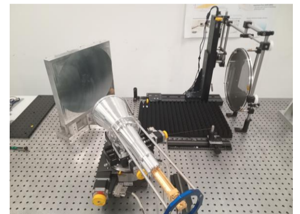
Bead pull setup for booster calibration
